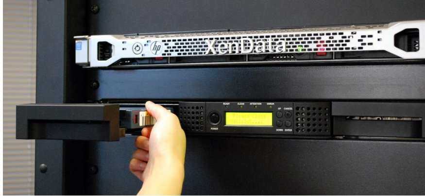
Data cartridges are exported from a robotic library via a 'mail slot'
