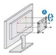
2. Attach the two slightly larger black screws to the bottom chassis cover of the X1.
