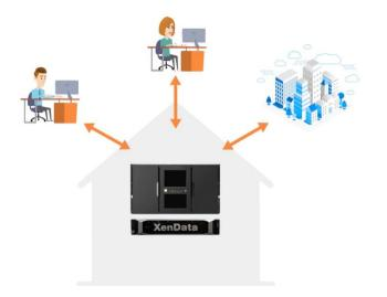
Adding an object storage S3 Server Interface to a XenData LTO archive system allows files to be written to and read from the archive from anywhere worldwide using fast and secure HTTPS. This option creates a private cloud interface. The on-premises interface and associated permissions are not affected: the LTO archive continues to be accessible locally using SMB, FTP or NFS.
