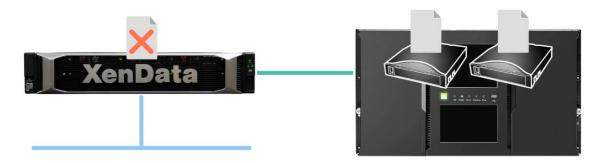
The stub file has the same properties as the original except the Microsoft offline attribute is set, indicating that the full file is no longer immediately available. Conversion to a stub file frees up space on the cache because the file representation on the disk is just a few Kilobytes in size.
