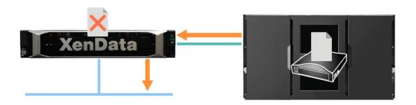
The case of a near-line restore from LTO is shown above. With LTO, near-line refers to a file that is a stub file on the disk cache, but it is stored on a cartridge within an attached tape library. The application that requests the restore issues a standard command to read the file. The XenData software will then cause the cartridge containing the file to be loaded into an available LTO drive and the drive then seeks to the beginning of the file. It is then restored to fulfill the read request.
