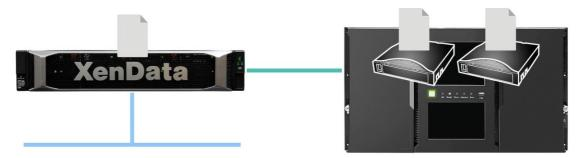
After the file has been written to a pair of LTO cartridges, there are three instances of it: two on LTO and one on the cache.
