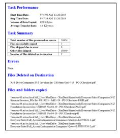
By enabling logging for an FS Mirror task, a log report is created each time the task is run. This can list all files copied, all deleted files and any files that were skipped due to being open. An example log report is shown here.
