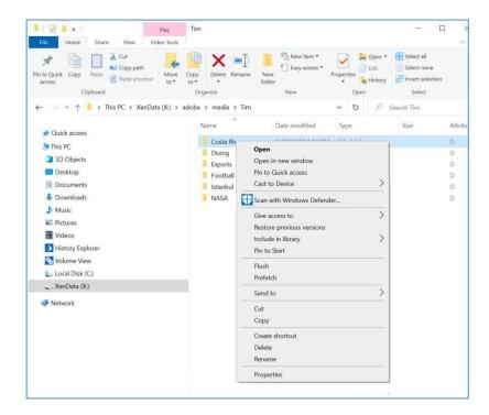
In this example, the entire folder 'Costa Rica' can be manually flushed or prefetched. Flushing is a quick operation that transitions all files in the folder and its sub-folders to near-line LTO. Of course, the system checks that all files are securely stored on LTO before flushing. Prefetch reads all the files from LTO and caches them on the managed disk. The prefetch operation reads all the files from LTO in the optimum order to minimize any unnecessary tape movement and cartridge swapping.
