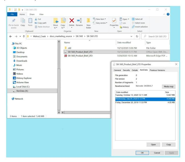
A similar process is used to restore deleted files, but because they do not appear in the normal file system, Windows File Explorer has been extended to include a History Explorer view of the file system which includes deleted files. History Explorer is launched from the left pane of File Explorer as illustrated above.
