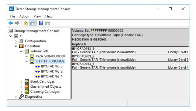
To access files stored on the legacy cartridges, a XenData catalog must be built first for each cartridge. This typically takes several hours for a full cartridge, as the entire tape must be scanned. After the catalog has been successfully created for a tape, the file and folder structure on that tape can then be made immediately available within the Windows logical drive letter managed by the XenData software. These operations are performed as follows for a single tape cartridge.
